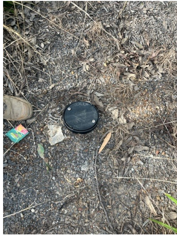
Photo 16: Groundwater monitoring well adjacent to the Tallawong Station car park
